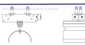
L: cable trolley length (mm). PL: diam. and useful width of the saddle (mm).
