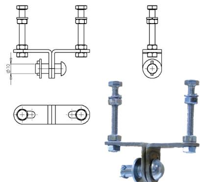
The clips makes a 90 degree turn in order to make easier the parking. When ordering, add to the reference, the necessary clips, followed by the indicative number: end clamp (-2), cable trolley (-5) or towing trolley (-6).
