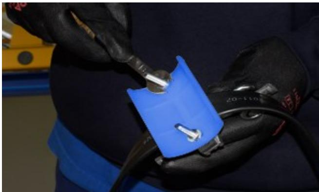
Tighten the screws of the cable holders avoiding damaging the cables due to excessive tightening. The cable package should be as centered as possible on the cable holder, so that the trolley runs in a balanced way. Make sure that the smallest cables do not slip into the cable package.
